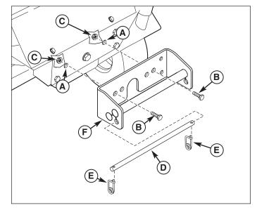
Figure 2. Front Weight Carrier Installation
